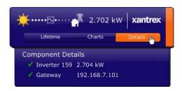
Component Details lists available devices on the Xanbus network, including the Gateway. Green check marks indicate devices that are online. The total power production of each inverter or inverter/charger is also listed in Component Details.
