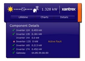
Click the name of the device with the fault to view the advanced diagnostic window and the fault/warning log for that device.
