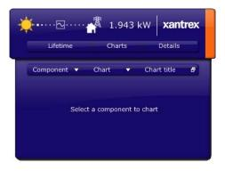
2. On the chart control bar, click **Component** and select the inverter for which you want to view charts. If you select **System Total**, the Widget displays charts showing data for the entire power system.
