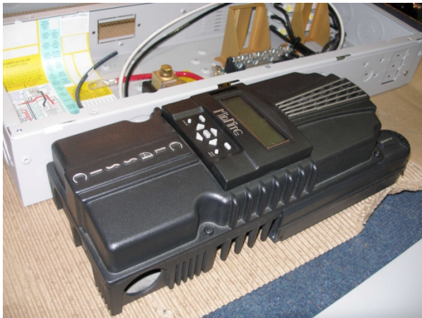
Figure 1.3D Classic mounted to the side of a MidNite Solar E-Panel
